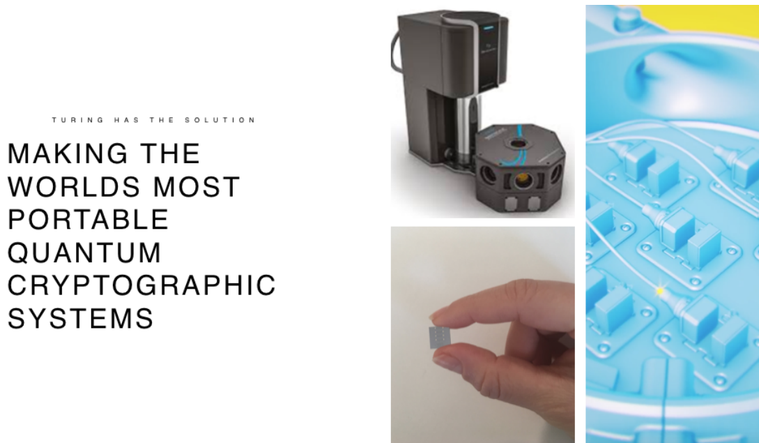
Figure 2: The Turing diamond based chipset within a portable 4K cryostat system. High operating temperatures and no vacuum systems makes the system significantly easier to physically move than architectures employing vacuums (Ion-Traps) or Dilution technology (Superconductors).
